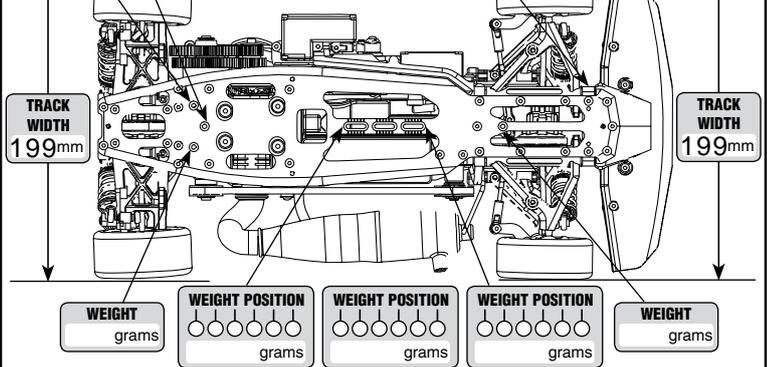
REMARKS Steering servo normal. Center block 3 point fixation.
