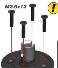
Do not overtighten the screws. There is always a gap between both sides of the diff housing.
