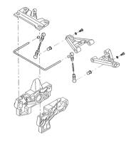
Softer rear anti-roll bars can be made by grinding a flat part of approx. 40mm wide on the anti-roll bar. The thickness of the anti-roll bar determines the stiffness.
