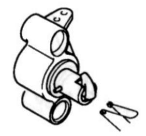
Place the nylon lever in the wheelaxle and press the steel 2.5mm pin through the hole. The lever pivots around the pin. Apply the torsion spring, the 2 legs snap behind the small edge inside the wheelaxle. Check that the axle turns freely with a minimal sideplay.
