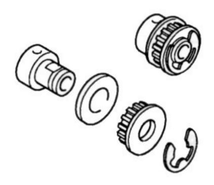
Press the 16T pully on the alu. pully adapter. Because of the small diameter of the pully the use of a cyano-glue or other strong glue is necessary to get a very firm and reliable joint between the pully and the pully-adapter. Secure the pully with the 7mm C-clips.
