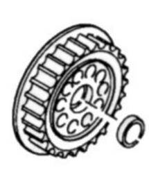
Remove the core from the 46T diff. pully. Press the 8x12mm ballbearing in the pully.
