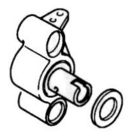
Insert the front wheelaxle and apply the nylon washer on the outside with the flat side of the washer facing to the outside.
