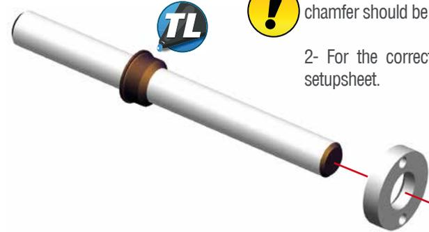
1- Notice that the piston is not symmetrical. The side with the chamfer should be assembled oriented to the shock shaft.
