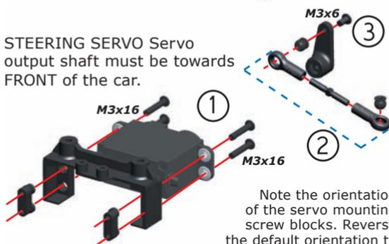
Note the orientation of the servo mounting screw blocks. Reverse the default orientation to mount a smaller servo.
